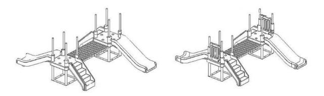
Place all the panels over the posts including the castle bridge walls and handrail of stairs and drill a Ø0,46in hole through post where stair handrail will attach. Attach stair handrails with hardware provided.
