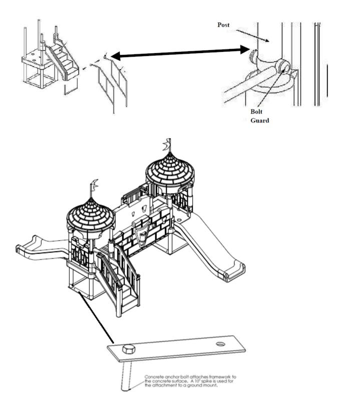
Secure structure to solid surface using anchor bolts, or secure structure to ground using 0,47 x 0,98in spikes. (Not provided)
